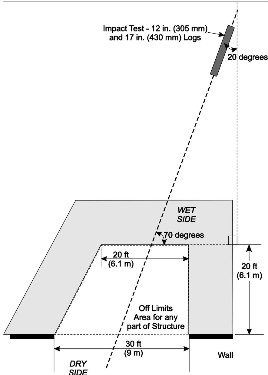
Figure 4.2.5.2 Debris Impact Test Layout
