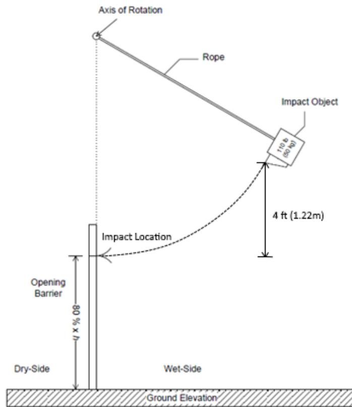
Figure 4.3.4 Impact Test Layout
